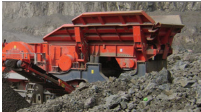
Hopper and Feeder
